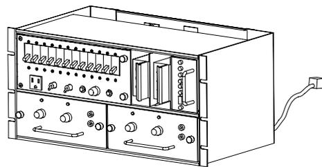
The PDA also houses two low voltage DC power supplies. One provides power to 24-volt devices, the other to 12-volt devices. Each of these power supplies is packaged as a slide-out subassembly.
