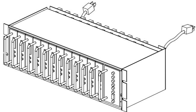
The detectors in the assembly can communicate to the controller in the form of either a contact closure or use of serial data strings. This will allow for the use of “smart” detectors that can pass additional information such as vehicle classification, Automatic Vehicle Identification/Location information, speed information directly to the controller unit, or video image-based detection units. Each slot provides general purpose power and input/output signals and a serial interface.
