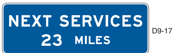
Figure 2E-43. Example of Next Services Sign
