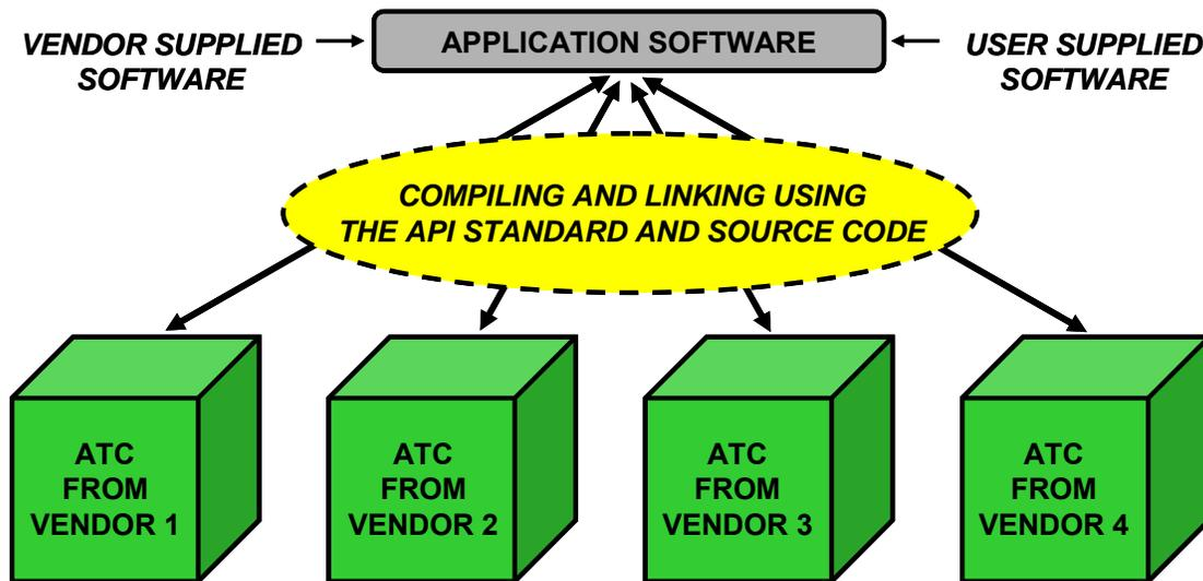
**Figure 2. Application program portability using the API Standard.**
