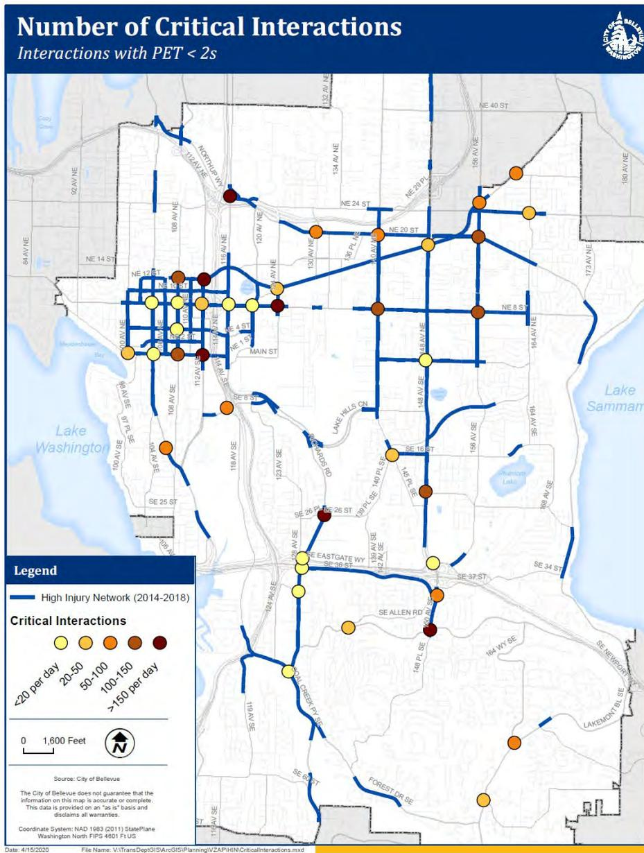
BriskLUMINA and BriskVANTAGE, products of Transoft Solutions, use artificial intelligence algorithms to process traffic camera footage to obtain traffic volume, road user speed, and near-crash event data. Results from the products are used to identify high-conflict interactions at intersections and to evaluate the efficacy of road safety improvements. Without improvements, these intersections are prone to future crashes.
